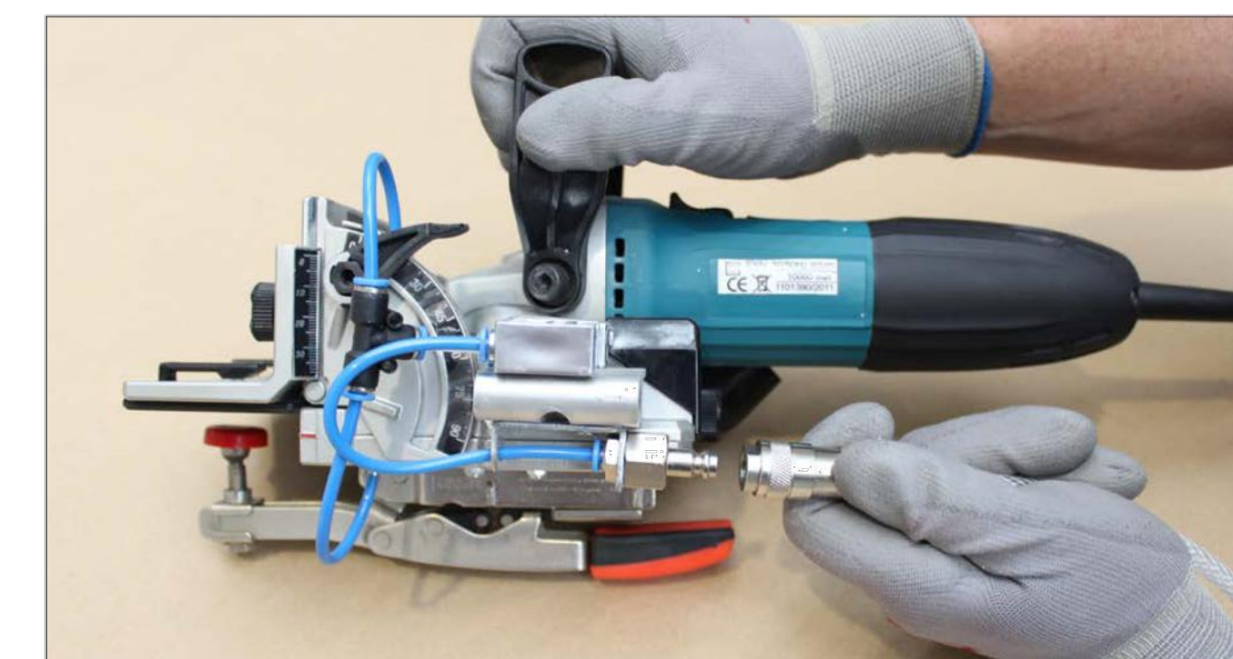
5. Turn tool on and check water cooling system works correctly.
