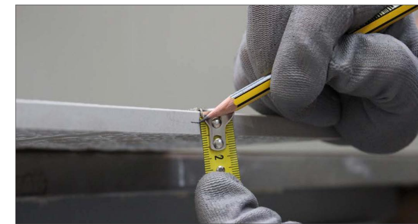
1. Make mark with position of kerf.
