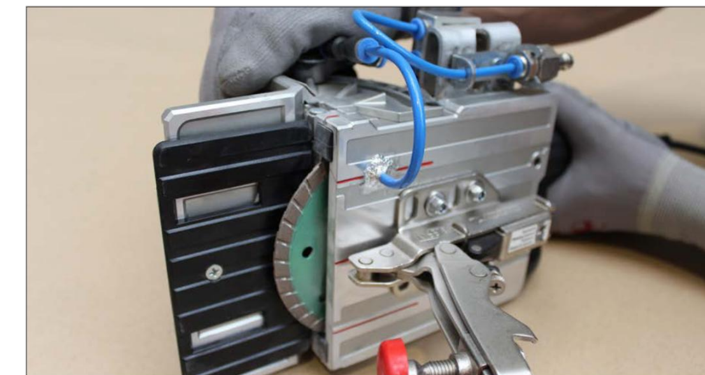
3. Check Blade is in Good Condition.
